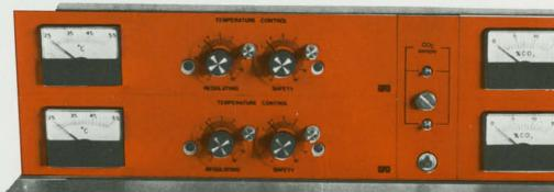
The Napco 7000 series are the only water jacketed automatic CO<sub>2</sub> incubator that actually tells you the temperature of the chamber, where your important experiment is taking place.
