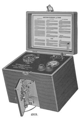
The temperature compensator is continuously adjustable in steps of  $5^{\circ}$  over the range 10 to  $40^{\circ}$ C. A zero adjustment is provided to compensate for changes in the asymmetry potential of the glass electrode. The walnut carrying case is  $11 \times 9 \times 8$  inches, with total weight less than 18 lbs. Closing the cover automatically shuts off the instrument and locks the door of the shielded electrode compartment.
